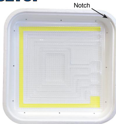
Unpack the incubator from the box. Remove the top half from the bottom. Lay the **Plastic Liner** in **Hova-Bator Bottom** then place the **Incubator Floor** on top of the **Liner**. Arrange the plastic floor as shown using the water troughs and turner power cord notch as reference. In most climates, fill trough #1 (highlighted in yellow) with water. Surface area, not depth, determines humidity; refill trough as necessary to prevent it from drying out.
